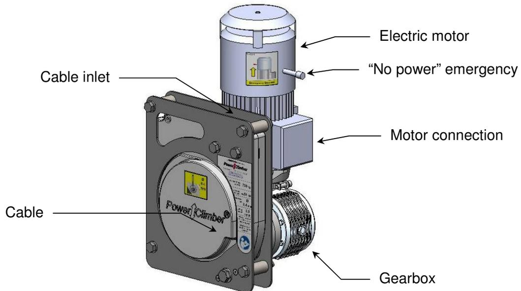
The ATLAS hoist is a self-reeving traction hoist, powered by an electric motor. The hoists and the central control box (CCB) are mounted on Temporary Suspended Platforms (TSP) and suspended with steel wire ropes from a suspension system. The strength of the platform and the suspension system used in combination with the hoists must be in relation to the Working Load Limit (WLL) of the hoist.
