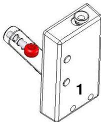
1. Insert the suspension rope through the eye of the slack rope lever.
