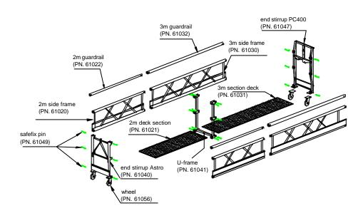
**Note:** Select the correct stirrup for use either with Astro or PC400/500 hoist.
